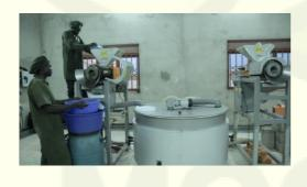
Cleansing and drying of the nuts before pressing
